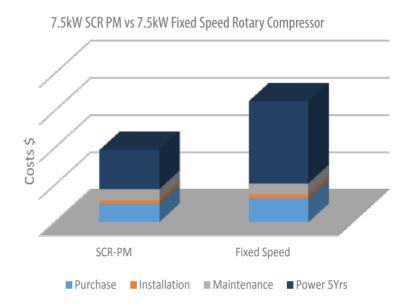
Chart compares the costs of owning a fixed-speed compressor to an SCR PM 7.5kw VSD compressor over just a five-year period, where the fluctuating air demand in a typical workshop, equates to a loaded run time of 30% of the day.
